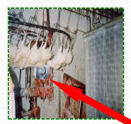
Poultry is transported on hooks through the slaughtering plant and after stunning the slaughter is performed by a rotating blade.
